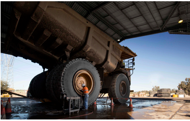
Figure 6. Ensuring all necessary tyre maintenance is performed while a haul truck is in the bay.
