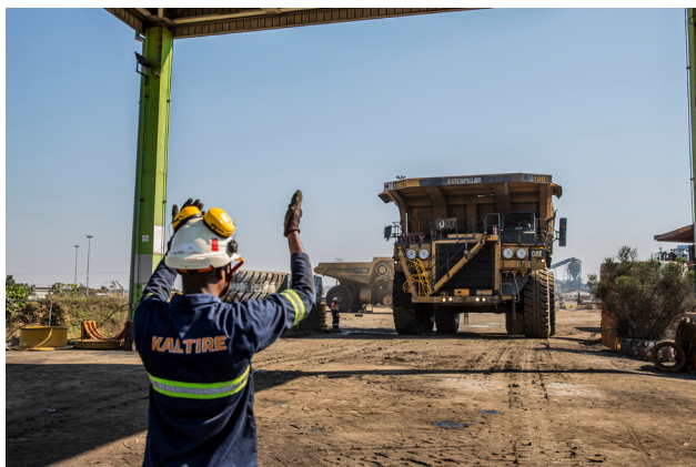
Figure 2. A team member directs a haul truck into the bay for tyre service.
