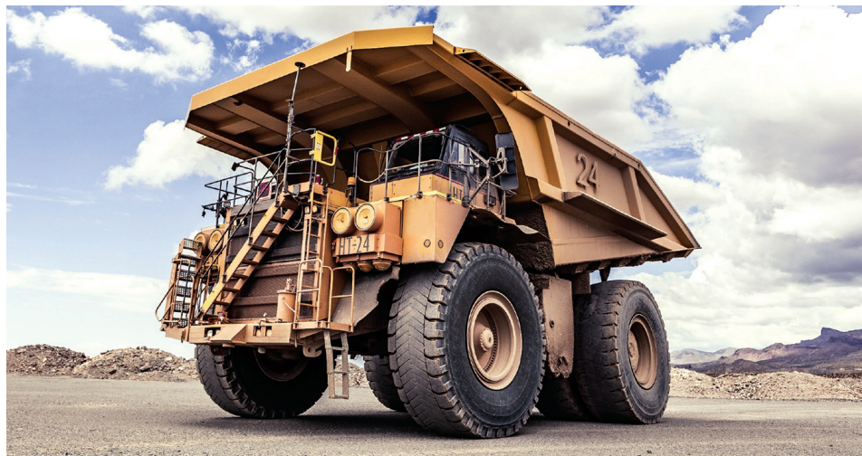
MasterCore is Bridgestone’s newest line of 57- and 63-in. tires for open-pit ultra-class haulage. (Photo: Bridgestone)
