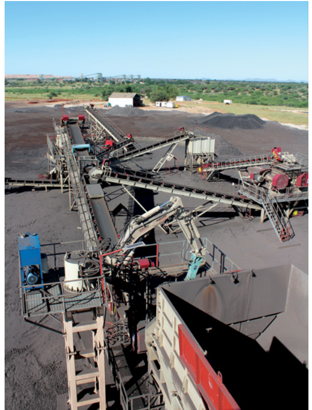
The mine uses a dry plant to process the manganese. The Kalahari is semi-desert and water scarce.
